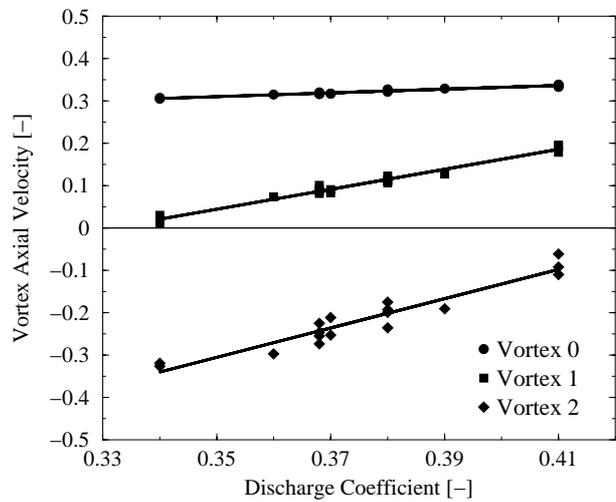
Figure 9. Characteristic axial velocities  $U_0$ ,  $U_1$ , and  $U_2$  versus discharge coefficient  $\varphi$ .
