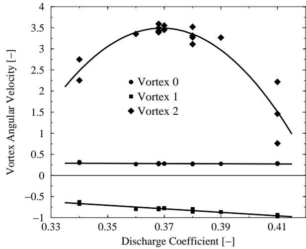
Figure 8. Characteristic angular velocities  $\Omega_0$ ,  $\Omega_1$ , and  $\Omega_2$  versus discharge coefficient  $\varphi$ .
