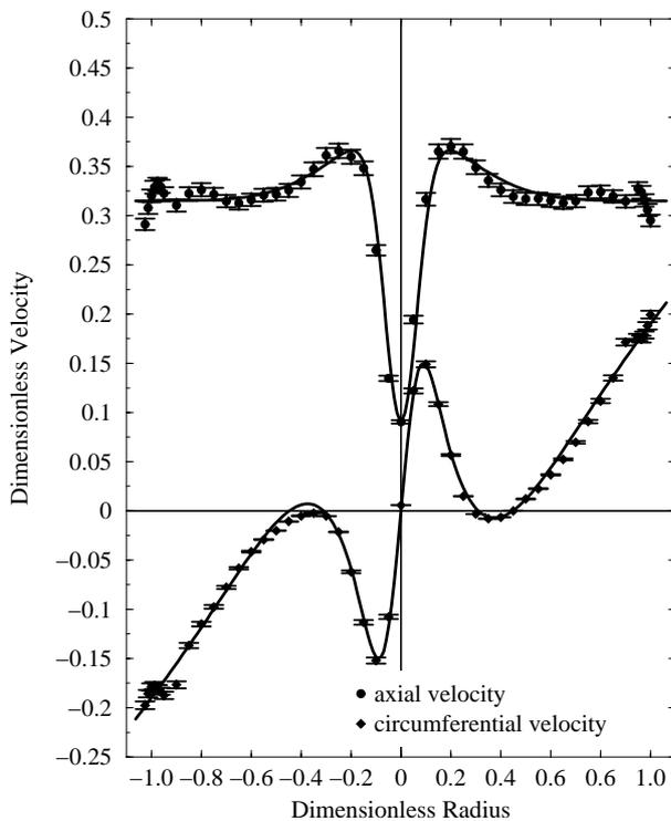
Figure 3. Axial and circumferential velocity profiles at discharge  $\varphi = 0.360$ .
