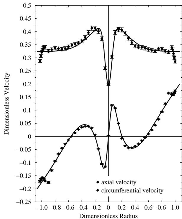
Figure 5. Axial and circumferential velocity profiles at discharge  $\varphi = 0.380$ .
