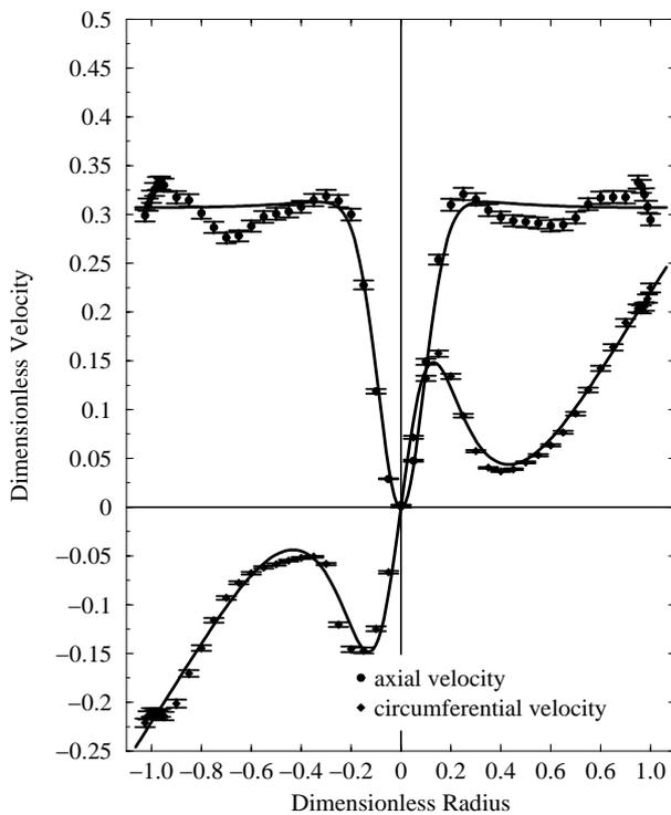
Figure 2. Axial and circumferential velocity profiles at discharge  $\varphi = 0.340$ .
