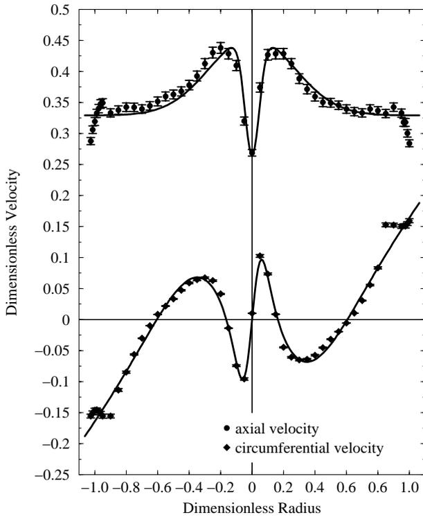
Figure 6. Axial and circumferential velocity profiles at discharge  $\varphi = 0.390$ .
