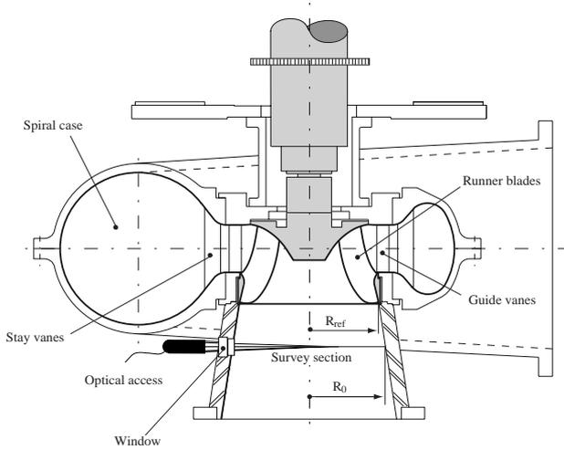
Figure 1. Sketch of the Francis turbine model and the LDA setup for the flow survey section at runner outlet.
