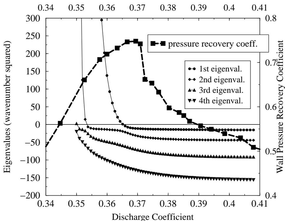
Figure 11. First four eigenvalues and the pressure recovery coefficient function of the discharge coefficient.
