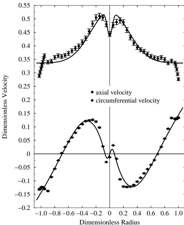
Figure 7. Axial and circumferential velocity profiles at discharge  $\varphi = 0.410$ .
