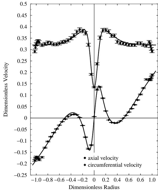
Figure 4. Axial and circumferential velocity profiles at discharge  $\varphi = 0.368$ .
